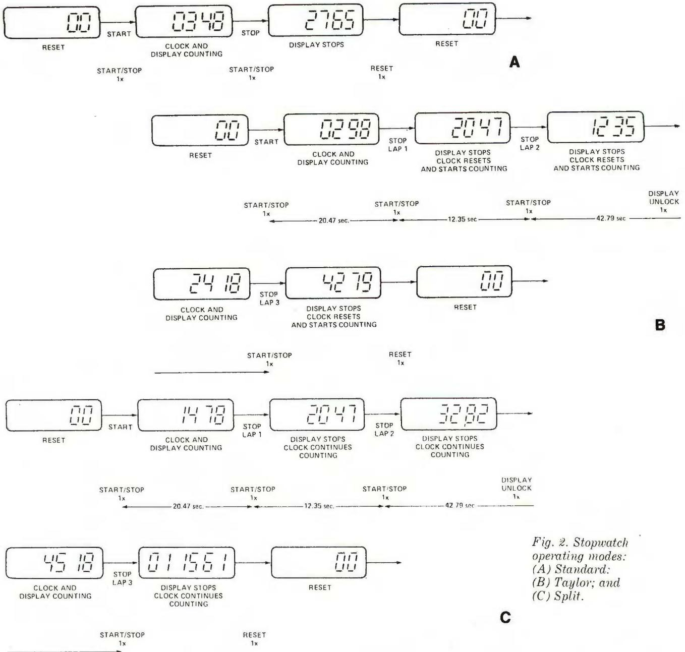
Fig. 2. Stopwatch operating modes: (A) Standard; (B) Taylor; and (C) Split.
