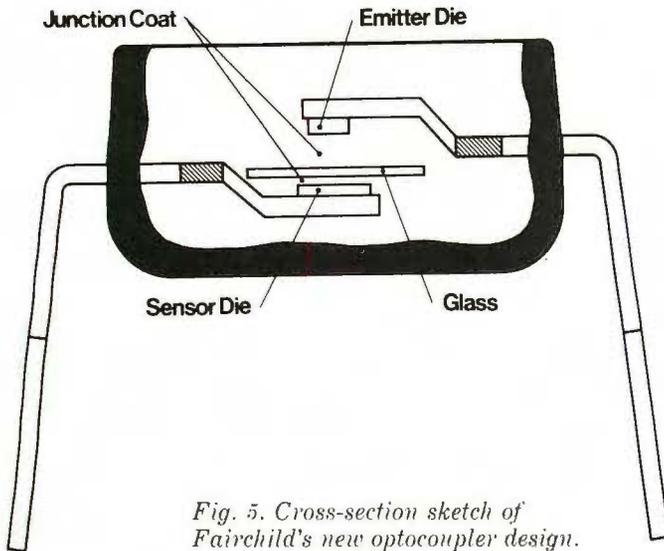
Fig. 5. Cross-section sketch of Fairchild's new optocoupler design.
