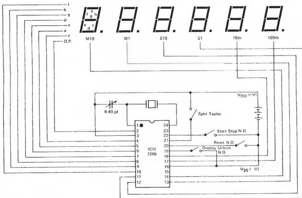
Fig. 1. Circuit for stopwatch using the 7205 chip.
